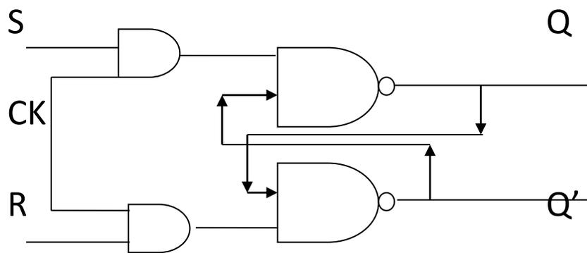
D flip Flop :- D flip flop is the enhanced version of Clocked SR flip flop. In SR Flip flop two input S and R are connected to an AND gate along with clock input. The output of each AND gate then applied to the NAND gate . The inclusion of clock signal ensure that the flip flop can be set or reset only when clock pulse is provided to the circuit.
