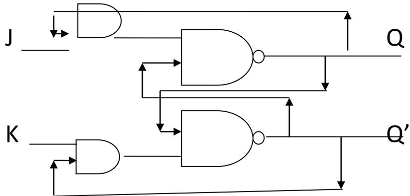
3. T- Flip Flop- T Flip-flop type is an enhanced version of the jk flip flop that accepts one input. Here, same input is applied in both the AND gate of jk flip flop. The truth table of T- Flip flop as :-
