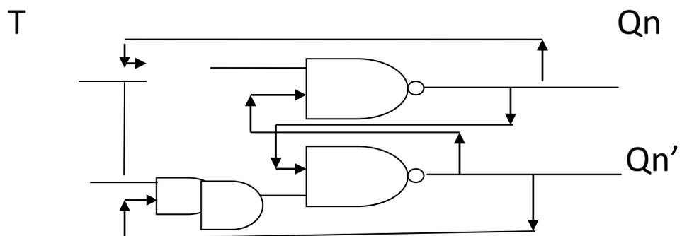
Clocked SR Flip Flop :- clocked SR flip Flop is built with a clock pulse to control the output of the SR Flip flop circuit. If the clock pulse (CK=1) its operation is exactly the same as SR flip flop. On the other hand when the clock pulse is not present (CK=0) the first gate are initiated i.e their output are 1 irrespective of the value of S and R. it means , the circuit responds to the input S and R only when clock pulse is available
